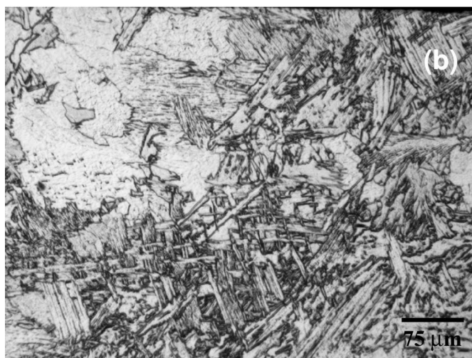
Figure 26 Optical micrographs showing the final microstructure at completion of each of the TRXRD experiments (a) in the HAZ and (b) in the FZ. The latter clearly shows two distinct morphological regions.
